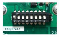
Set the channel on the dip switch like on all receivers on the layout.
