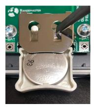
To check the batteries voltage, please use voltmeter and test the battery level while pushing the button. If it is lower than 4V, please exchange the battery:
