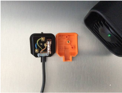
Triple core cable with 0.75mm 2 cable diameter
