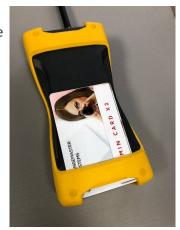
To enter administration section attach the admin chip card to the back side of the device.
