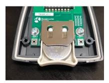
In order to make sure that contact of the batteries is good, every time when changing the batteries, please push the connecting parts of the battery holder inside:
