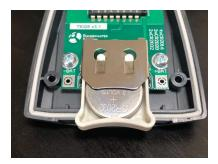
In order to make sure that contact of the batteries is good, every time when changing the batteries, please push the connecting parts of the battery holder inside:
