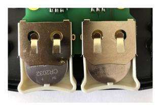
To check the batteries voltage, please use voltmeter and test the battery level while pushing the button. If it is lower than 4V, please exchange the battery!
